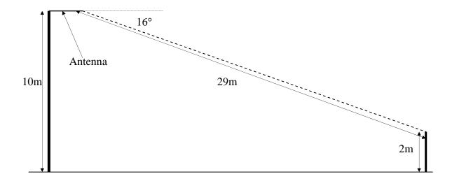
Note that there will be sidelobes off the boom axis. Due to the low gain in these lobes, the minimum separation distance in these directions would normally be met at a distance less than eight metres and can be ignored. However, if there are sidelobes with significant gain they may need to be considered.
